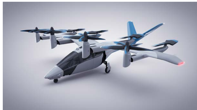
Vertical Aerospace's VA-X4 has a winged design that gives it lift and reduces electrical load when in flight.
